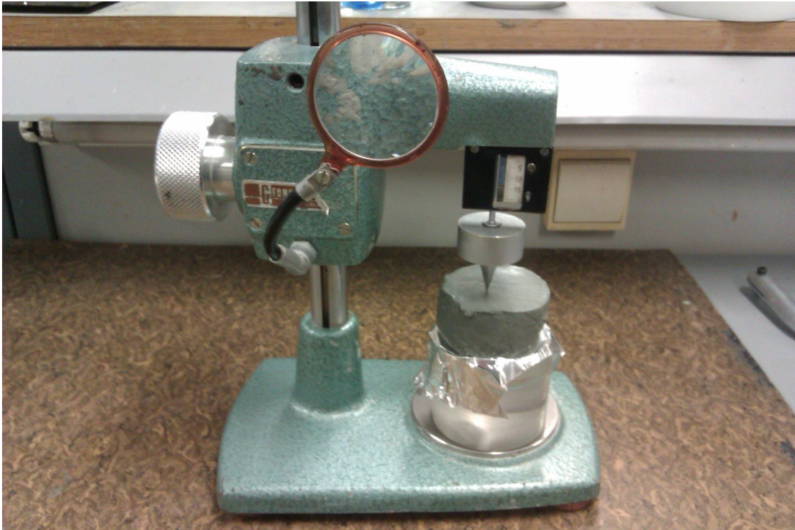
Figure 3.9.1: Falling cone test apparatus with mounted cone and undisturbed sample.
