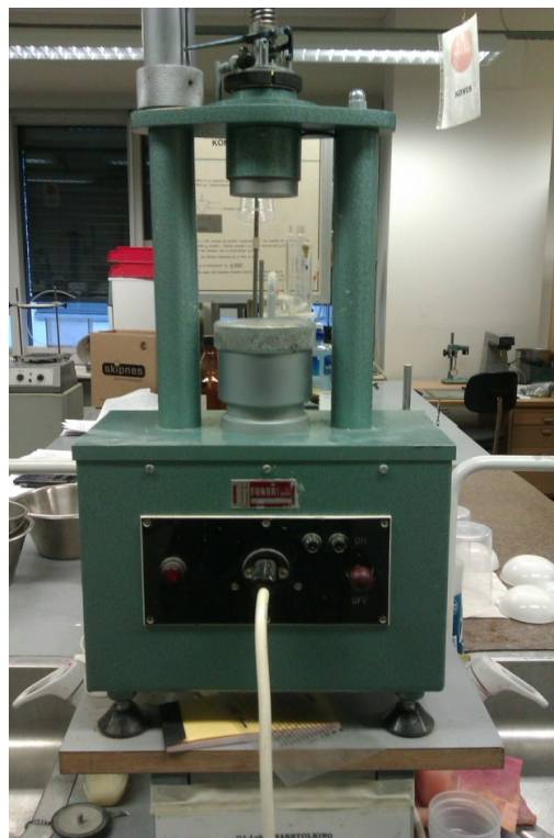
Figure 3.8.1: Unconfined compression test rig used in the study.
