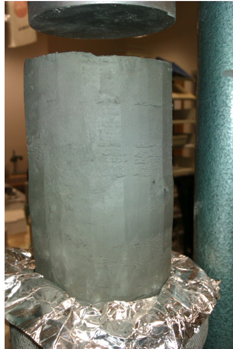
Figure 4.3.4: Sample T2-H15: Specimen at the end of UCT.
