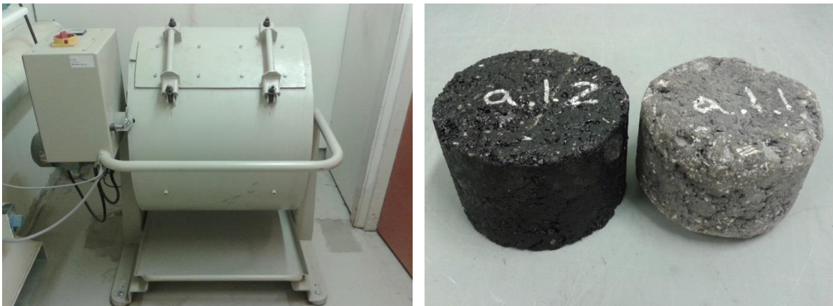
Figure 12: Los Angeles machine and specimens before and after the Cantabro test
