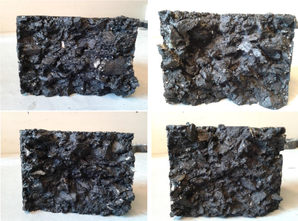
Figure 38: Aggregate coating. From left to right: Steinkjer and Vassfjell on top, limestone and hydrated lime on the bottom
