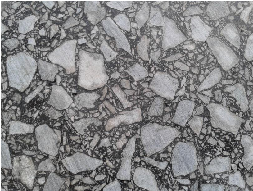
Figure 39: Saw kerf surface for evaluation of the aggregate coating
