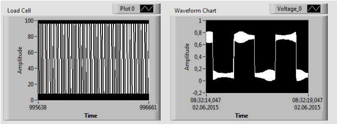
Figure 17: Variations in the applied load pulse due to noise in the system
