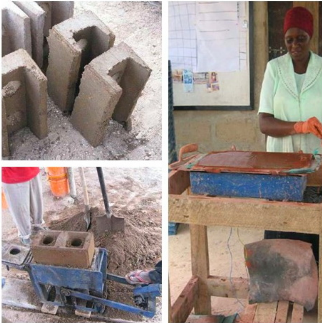
Figure 4.4: From the left counter-clockwise: Special bricks used above windows and doors, photo by: Qidi Jiang, 2013 /Making of a typical inter-locking brick, photo by: Qidi Jiang, 2013 /Making of a roofing tile, photo by: Margaret Ricke, 2011
