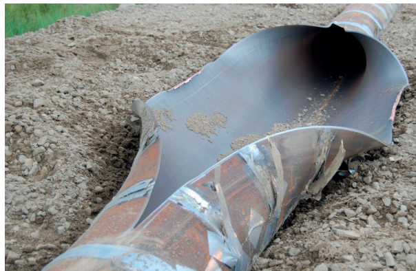
Figure 1.1: A pipe after a crack has propagated. Credit: SINTEF Material and Chemistry.
