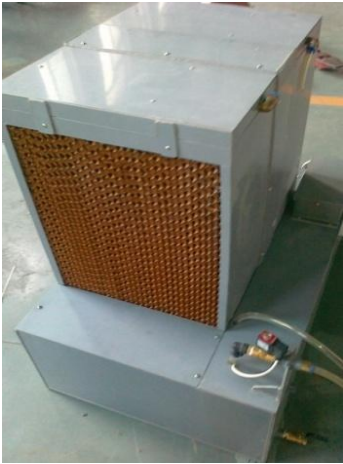
Figure 26: The cross-flow direct evaporative cooler
