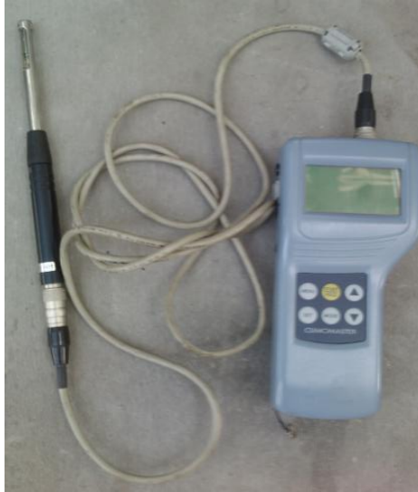
Figure 45: The CF8585-model TSI anemometer
