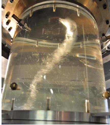
Figure 3.2-1 – Draft tube or Rheingans vortex at the Waterpower laboratory
