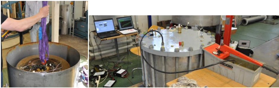
Figure C.2 Runner installation (left) and overview of calibration setup.
