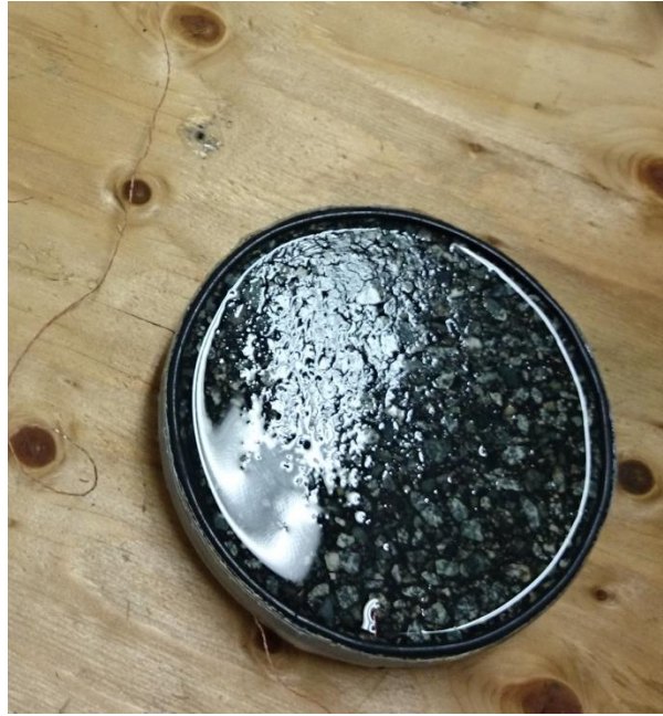
Figure 8 Substrate 24 hours after spraying of NaCl in the ice laboratory
