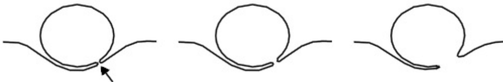
Figure 2.4: First, a small hole is formed in the film. The interfacial tension is immediately acting to minimize the film surface area and hence expands the hole which eventually will lead to collapse of the droplet
