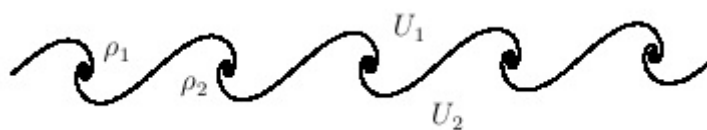
Figure 2.5: A parallel stream with the heaviest fluid on the bottom \rho_2 > \rho_1 and the with a relative velocity difference U_1 > U_2
