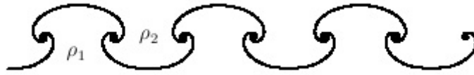
Figure 2.6: Parallel stream with the heaviest fluid on top \rho_2 > \rho_1 . As the instability develops, perturbations are rapidly amplified into penetrating Rayleigh Taylor fingers and a very distinct mushroom cape is formed
