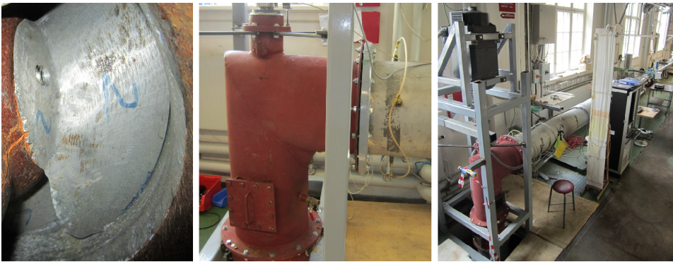
Figure 2.9: Runner vane with four settings - 90 degree bend before turbine - The generator is placed on top of the turbine
