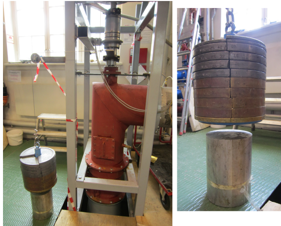
Figure 4.2: Calibrating the torque transducer
