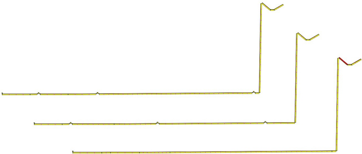
Figure 7.3: Simplified Girassol geometries. Pressure profiles at riser inlet shown in Figure 7.4. Pipe diameter rescaled by a factor 75
