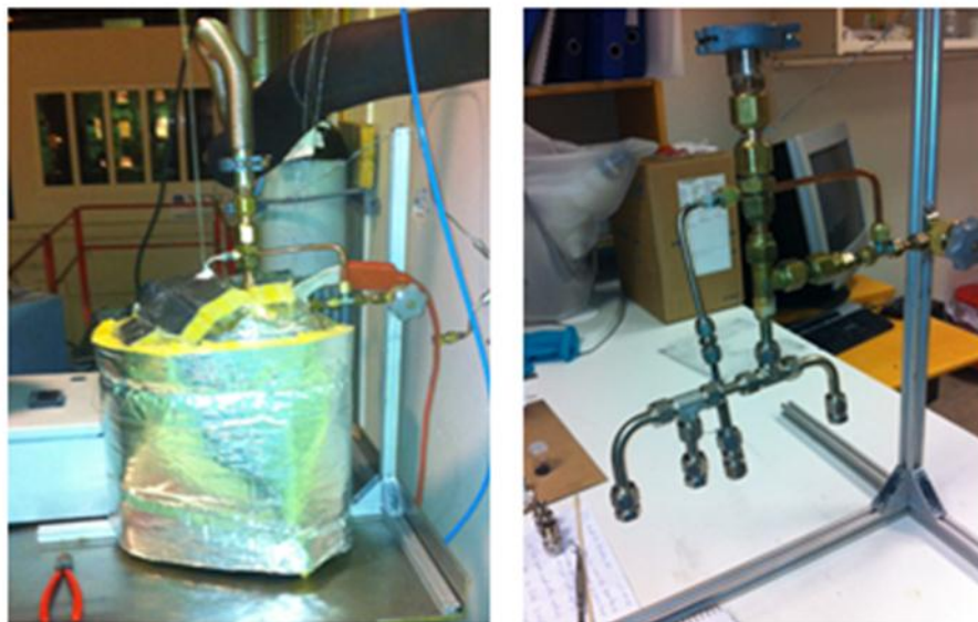
Figure 3-3: The activation set-up. (Left) Activation in process with heating band, isolation and connected to the vacuum pump. (Right) Show the pipe set-up with its corresponding four metal end caps.
