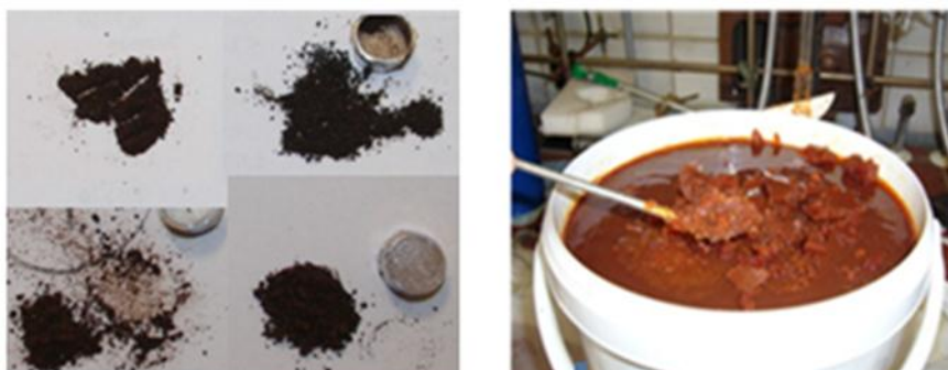
Figure 4-16: Fe-btc activated samples; the difference between the 1. set (up) and the 2. set (down). (Right) The Fe-btc inactivated gel.
