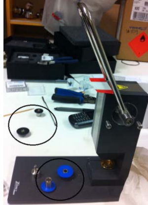
4-2 The Tzero® sample press with its belonging blue and black press parts.
