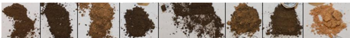
Figure 4-21: MIL-100(Fe) activated samples; the four first ones from the left are set 1, the next three samples are set 2, all in chronological order according to the experimental sequence, and the last one is an inactivated sample.
