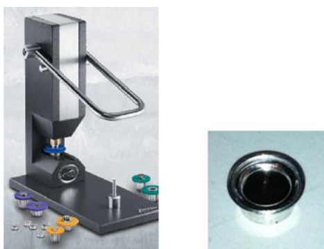
Figure 3-2: (Left) The Tzero™ press with its corresponding encapsulation parts [37]. (Right) An encapsulated sample with Tzero™ pan and hermetic lid.
