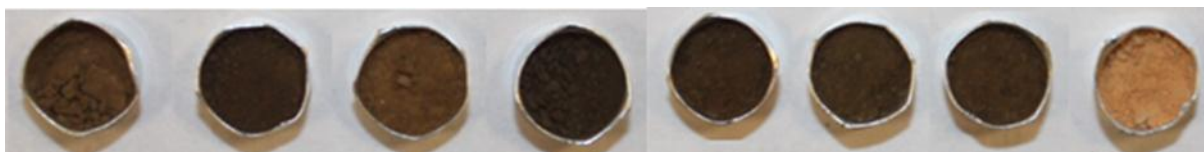
Figure 4-20: MIL-100(Fe) activated samples; the three first ones from the left are set 1, the next four samples are set 2, all in chronological order according to the experimental sequence, and the last one is an inactivated sample.
