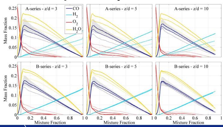
The objective was to investigate the influence of H<sub>2</sub> content in fuel and jet Reynolds number on localized extinction and flame structure
