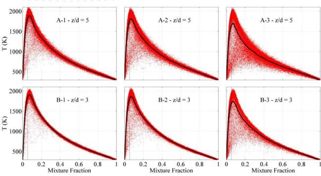
Leads to local temperatures drops due to increasing heat removal rates from convection and diffusion along with decreasing chemical reaction rates.
