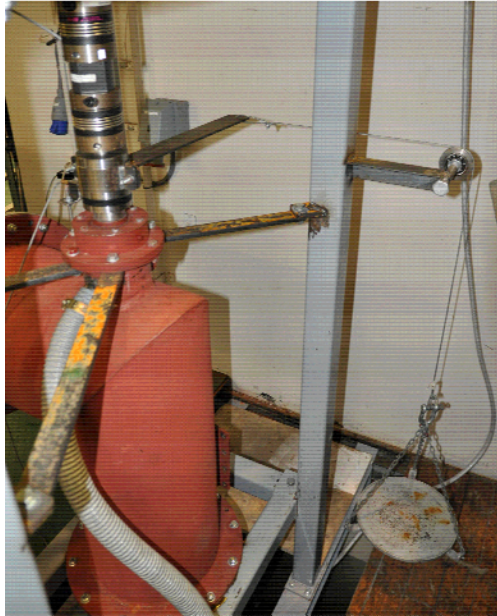
Figure 3-3 The dead weight calibration setup
