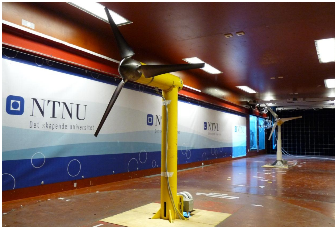
Fig. 4.2: The two model wind turbines set up in the wind tunnel of NTNU
