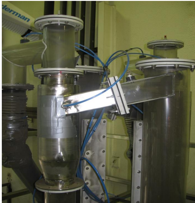
Figure 3-10: Picture of the Cyclones which are used in the Cold Flow Model rig
