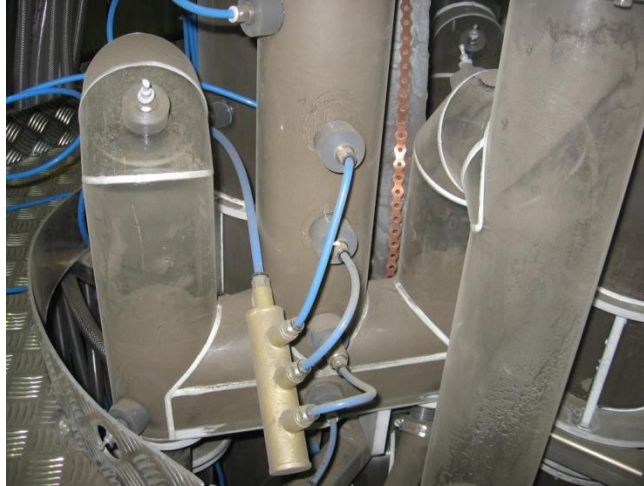
Figure 3-9: On site picture of loop seal which is used in Cold Flow Model rig
