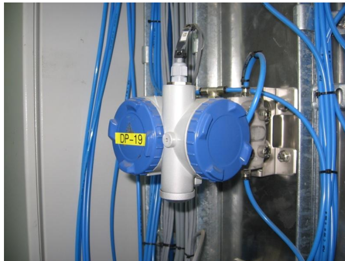
Figure 4-8: Picture of the pressure transmitter which are in used in the Clod Flow Model rig
