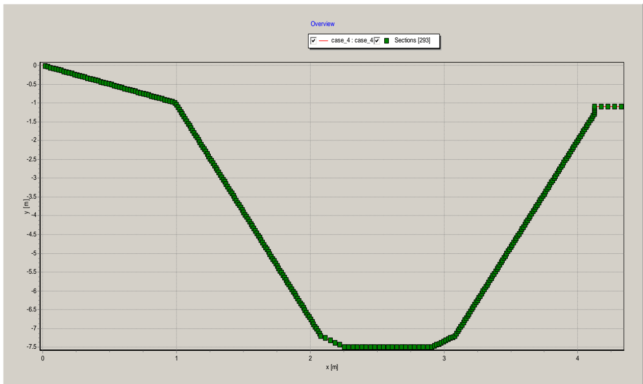
Figure 22 L-riser geometrical description in OLGA
