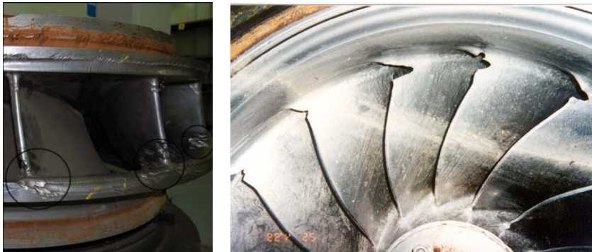
(a) Erosion damage at runner inlet, Cahua power plant [12] (b) Erosion damage at runner outlet, Jhimruk HEC [11]
