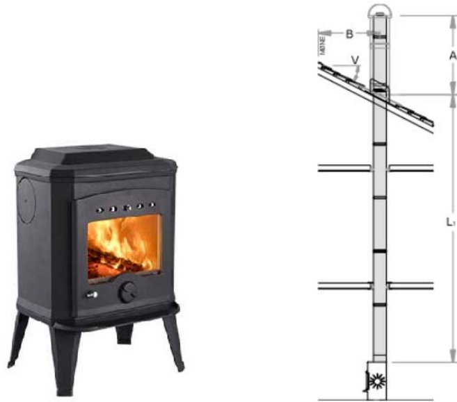
Figure 2.11: Left: Photo of the wood stove “Saturn”. Right: Illustration of a Nordpeis stove and chimney installed in a two floor high residential building [22].
