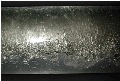
Figure 7.1 Stratified oil-water flow in a 0.056m pipe ( u_{\text{mix}} = 1 m/s, input water cut is equal to 25%).
