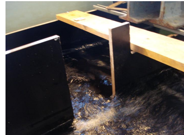
Figure XII-21: First attempt to regulate the flow rate in the channel. Strong non-uniformities and vortices in the flow are visible.
