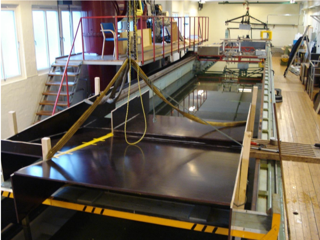
Figure XII-13: Model over the tank during the installation phase
