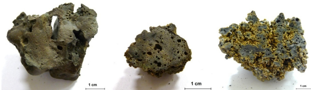
Figure 7-2 Sectional area of the sintered ash from combustion of wood pellet (left) and mixed with 4 (middle) and 8 percent sewage sludge (right).
