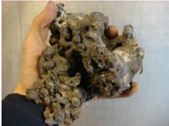
L.1 Sintered and agglomerated ash lump
