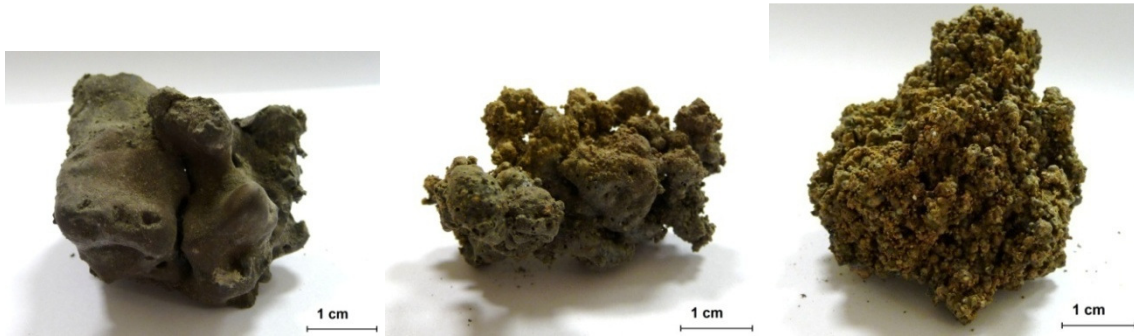
Figure 7-1 Pictures of sintered ash after combustion of pure wood pellet (left) and mixed with 4 (middle) and 8 percent sewage sludge (right).
