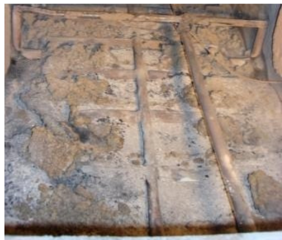
L.4 Ash after combustion with 8 percent sewage sludge
