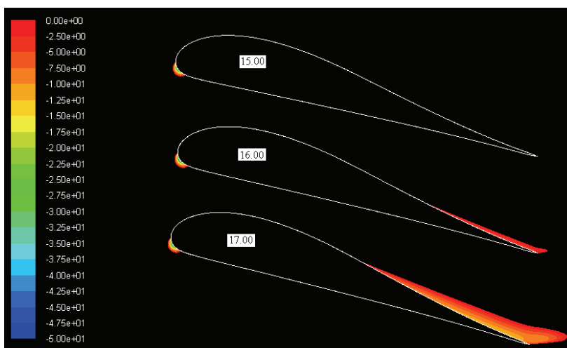
Figure 5.5.4 – B1, reversed flow, CFD simulation.
