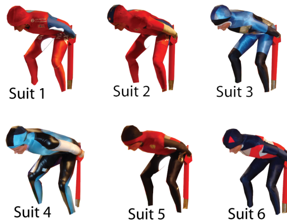
Figure 10.2: A picture of the 6 suits tested. All the suits have different patterns in the different parts of the body. Suits 1,3,5,6 have a moderate rough textile on their legs while suit 2 has an extreme rough pattern and suit 4 is totally smooth.
