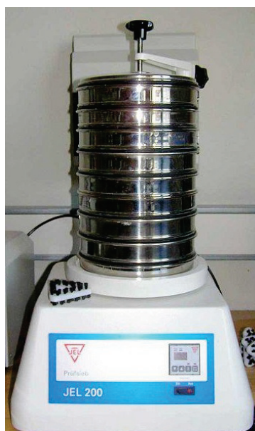
Figure A.1: Sieving analysis equipment.
