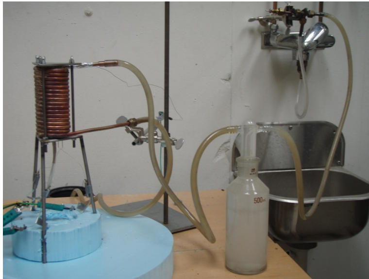
Figure 4.4.: Tap Water Cooling
