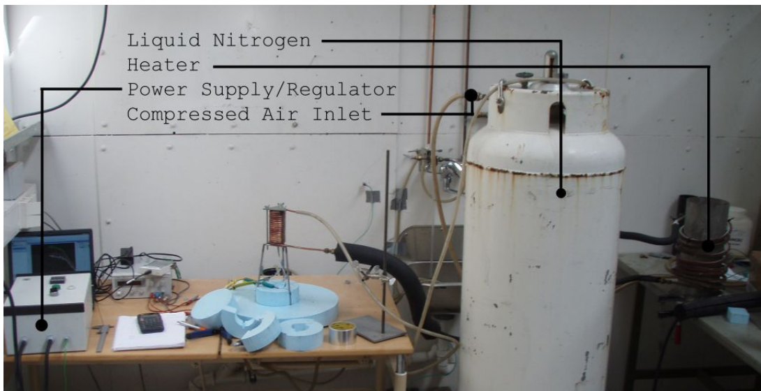
Figure 4.6.: Liquid Nitrogen Coolant Setup
