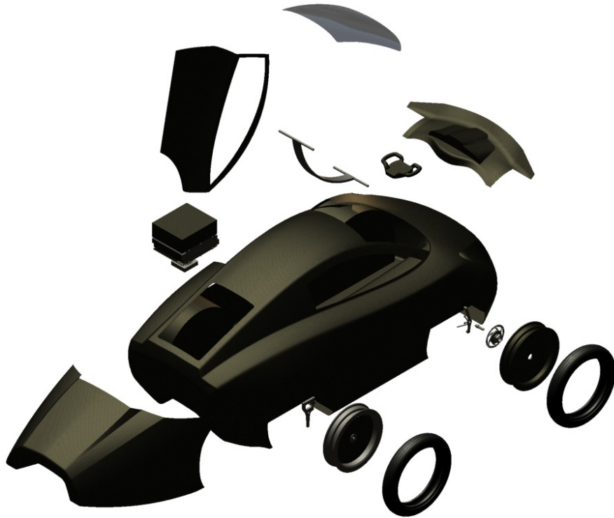
Figure 4.16: Exploded view of DNV Fuel Fighter 2010.
