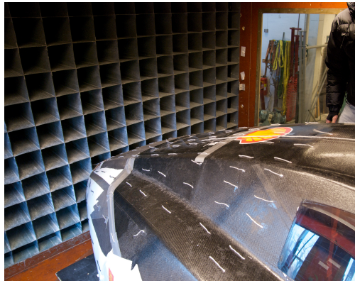
Figure 4.7: The rig was positioned at the rear most position in the wind tunnel, which could affect the wake and hence the drag measurements of the car.
