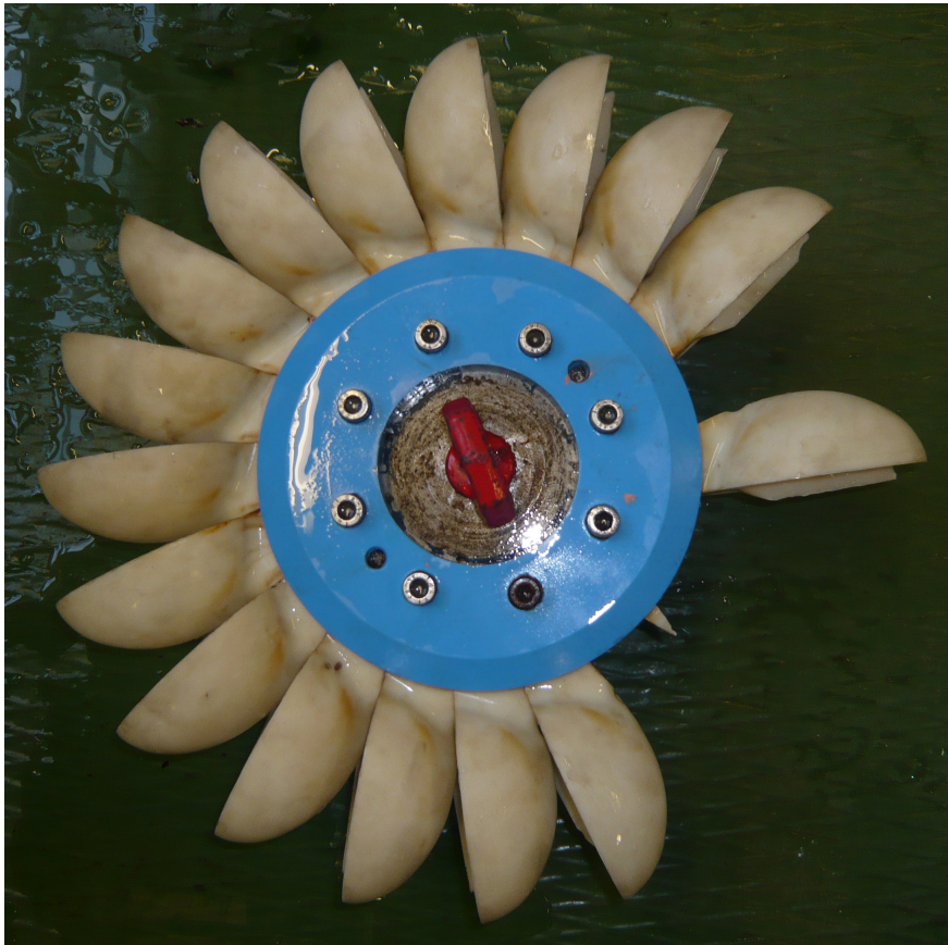
Figure E.6: The turbine after it was taken out
