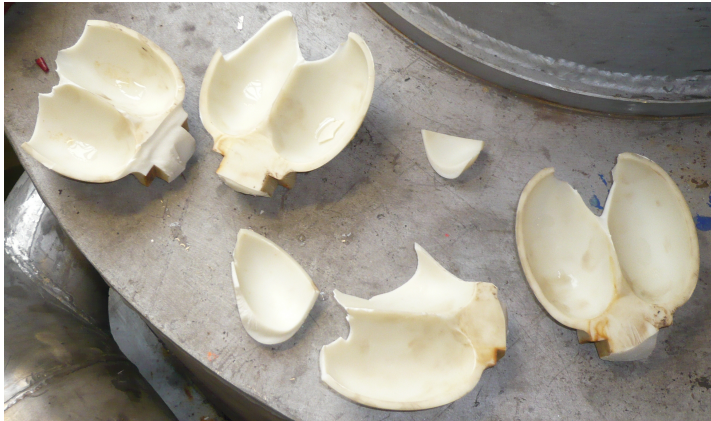
Figure E.4: The 4 buckets that were broken off the turbine by the rings
