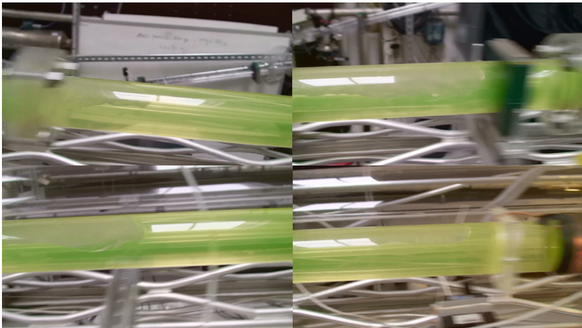
Picture D 4. U_{sl} = 0.64\text{m/s} , .5-degree inclined. T-L: 4m; T-R: 6m; B-L: 11m; B-R: 13m.
