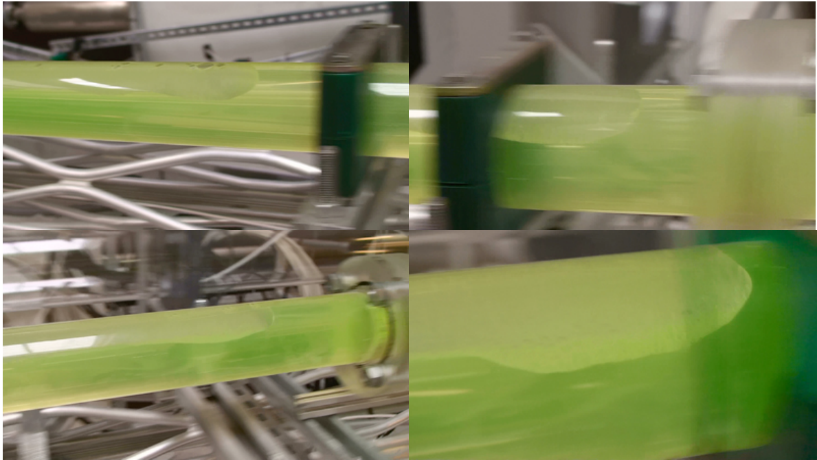
Picture D 3. U_{sl} = 0.49\text{m/s} , .5-degree declined. T-L: 4m; T-R: 6m; B-L: 12m; B-R: 13m.
