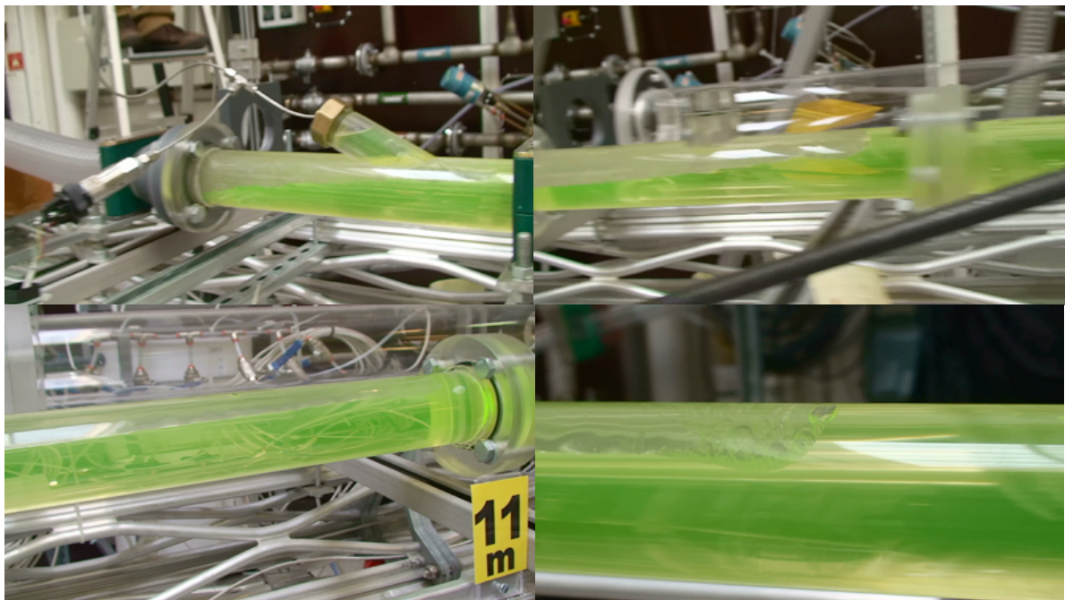
Picture D 2. U_{sl} = 0.23\text{m/s} , .5-degree declined setup. T-L: inlet; T-R: 1m; B-L: 11m; B-R: 13m.
