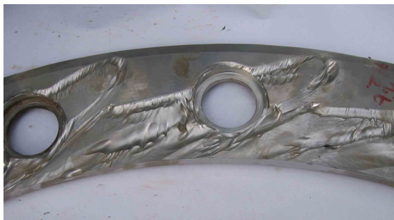
Figure 5.5: Eroded guide vane cover[Dah]
