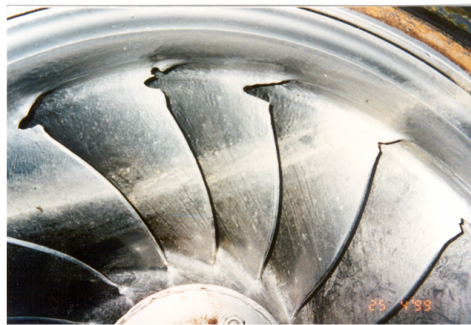
Figure 6.6: Damage of runner outlet[Dah]
