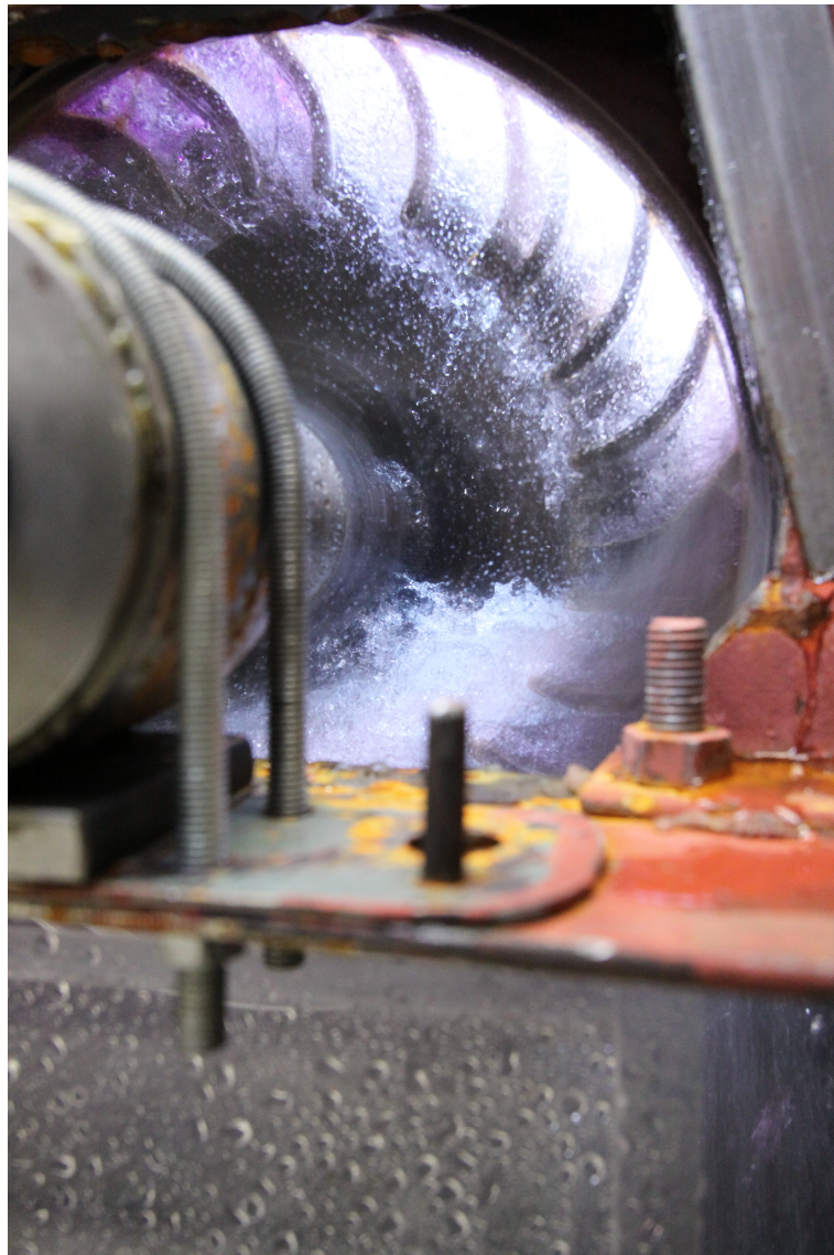
Figure K.1: 20% nozzle opening at a rotational speed of 350 rpm
