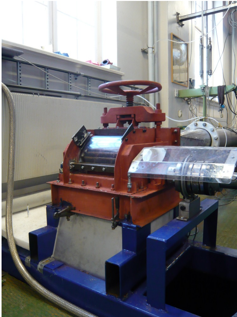
Figure L.2: The cross-flow turbine after remodeling
