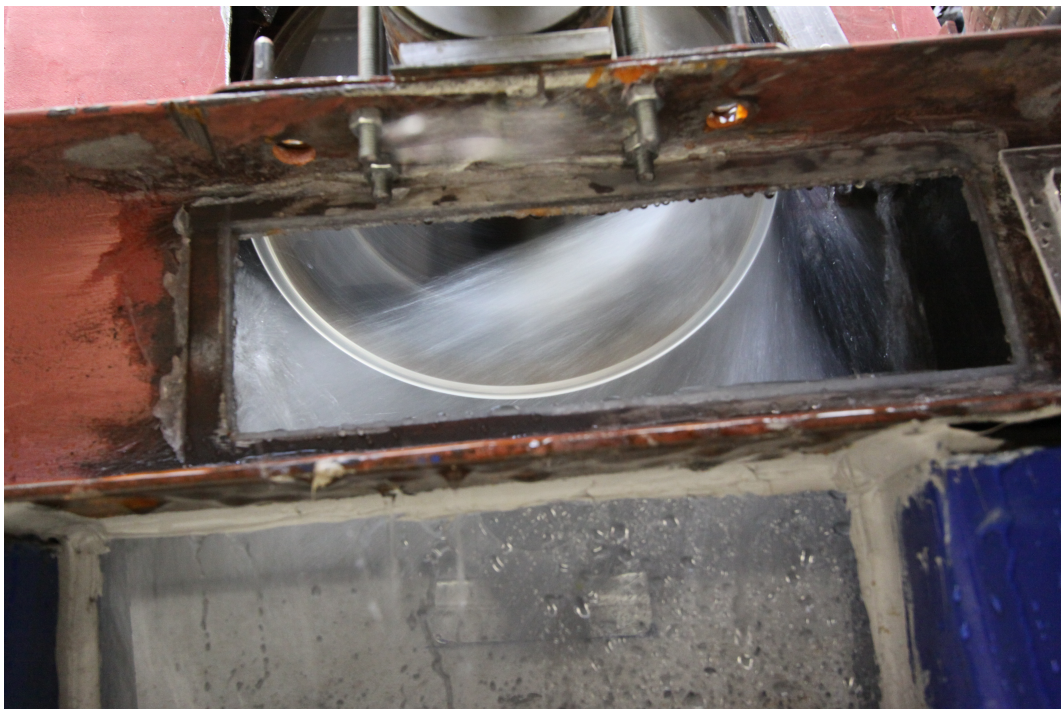
Figure K.2: 20% nozzle opening at a rotational speed of 350 rpm
