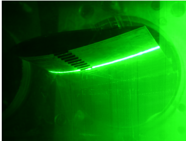
Figure 3.7: The laser plane and the NACA0015 hydrofoil
