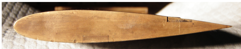
Figure 3.1: The NACA0015 hydrofoil made in brass used in this project
