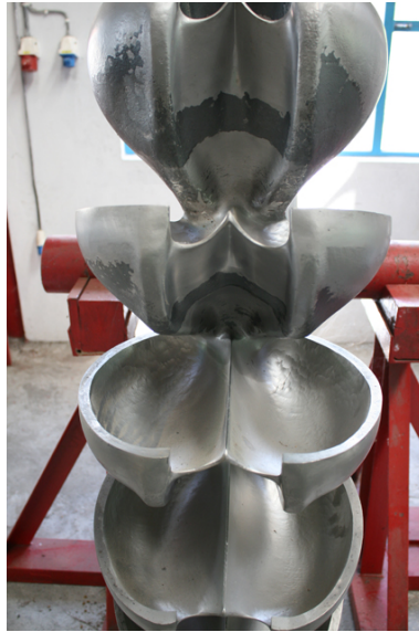
Figure C.2: One of the runners at Khimti, ready for maintenance.
