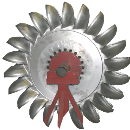
Figure 2.19: One of the old pelton runners at Khimti I.
