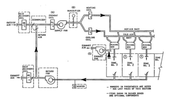
Figure 16 Air mixing system (DDS, Dual-Duct System) [8]
