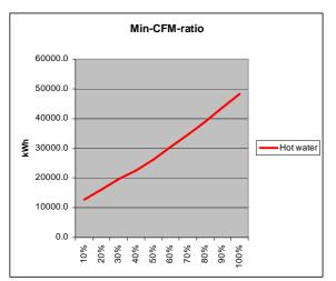
Figure 49. The affect on hot water demand when changing the minimum cfm ratio in the system terminal boxes of Case 3.
