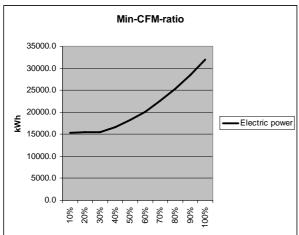
Figure 50 The affect on electric demand when changing the minimum cfm ratio in the system terminal boxes of Case 3.
