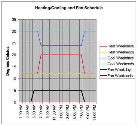
Figure 30. Heating/Cooling and fan schedule. The fan is turned on at 5 AM and off at 8PM.
