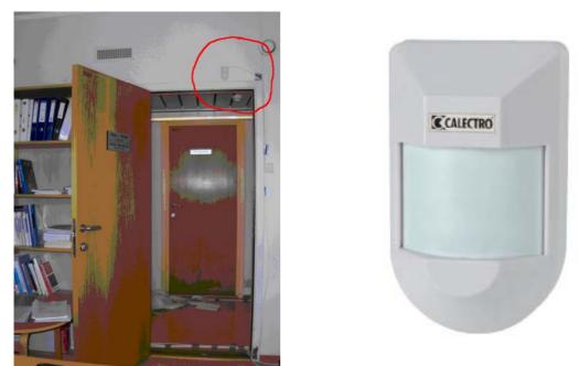
Picture 5. Left; Mounting of the SWE-V sensor over the door. The picture is taken from the workspace. Picture 6. Right; Calectro model PIR-TF-25. Wall mounted infrared motion sensor. Named SWE-V in this thesis.
