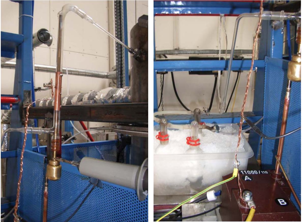
Figure 3-3: The nonthermal plasma reactor, the outlet from the macro-TGA (left) and the inlet to the condensation bottles (right).
