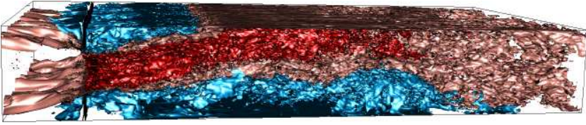
FIGURE 2.1. Instantaneous streamwise velocity field for turbulent flow over slits (see paper 8). The red iso-contours indicate positive velocity regions while the blue represent negative velocity (i.e. recirculation bubbles).
