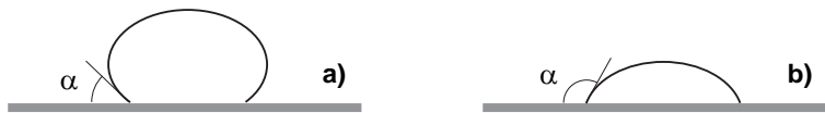
Figure G3 Principle of water bubbles on a non-wetting (a) and a wetting (b) surface. \alpha is the contact angle of the bubbles.
