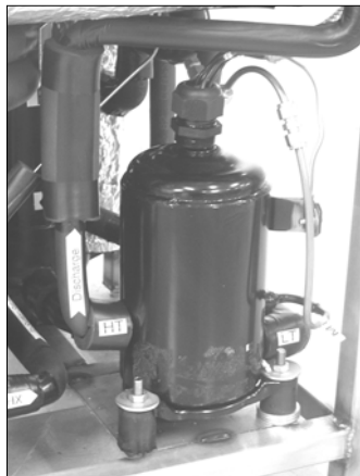
Figure 4.5 The Sanyo two-stage rolling piston compressor (prototype).
