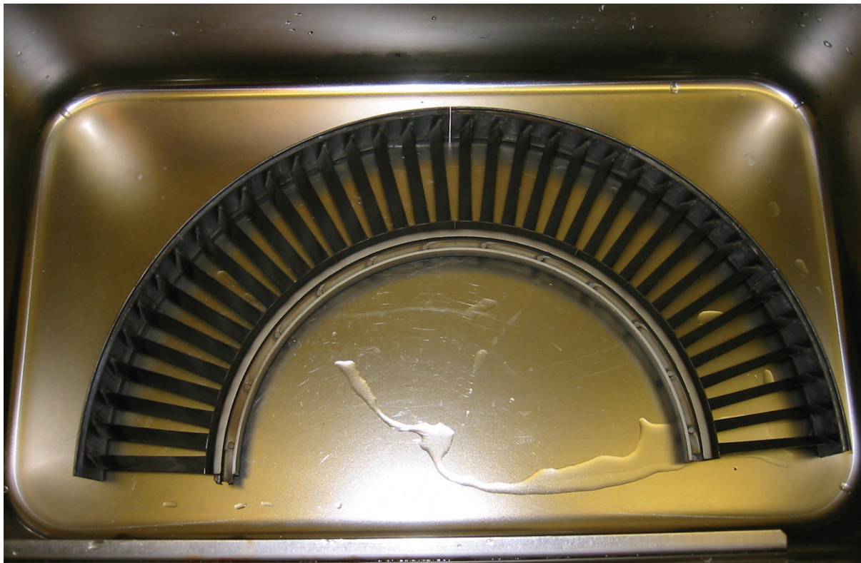
Figure 25 Dissolving salt on the first stage stator vanes
