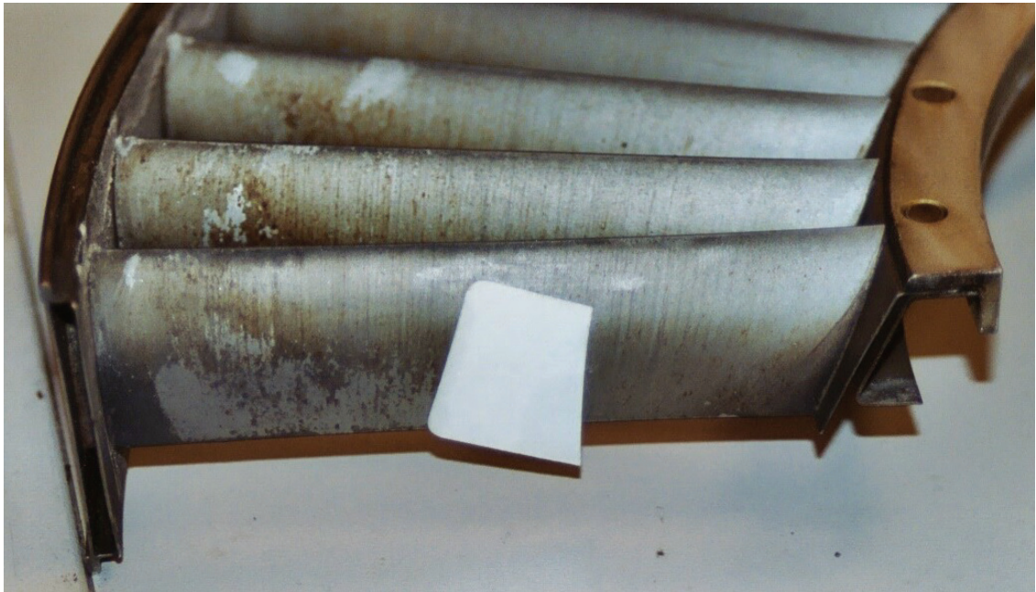
Figure 24 Application of Struer's replicas to collect salt grains (first stage suction side)
