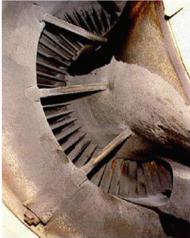
Figure 1 Example of heavy dust fouling in axial compressor [62]
