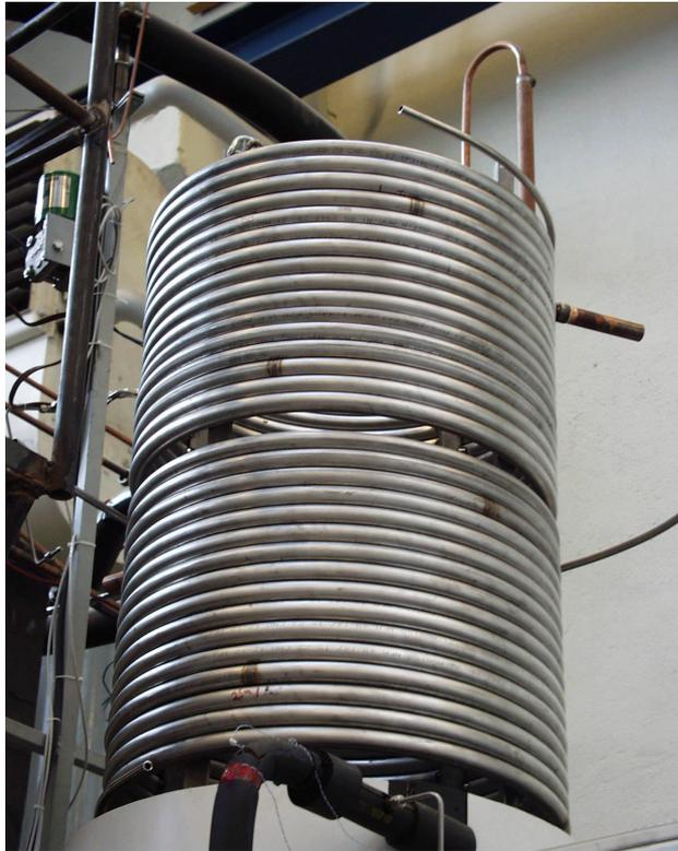
Figure 4-7 The heat rejecting heat exchanger
