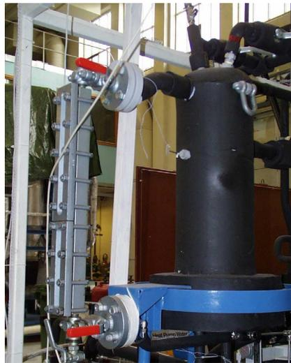
Figure 4-9 Integrated liquid receiver/submerged heat exchanger
