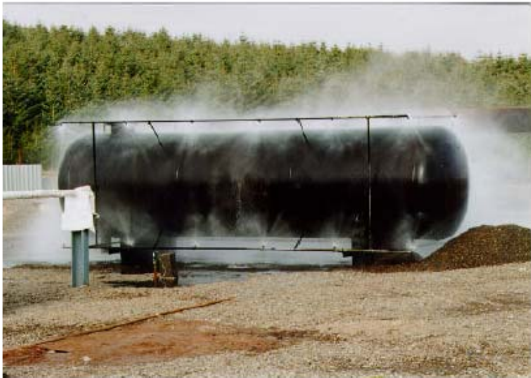
Figure 3.5: Water spray nozzles deluging the target [92]
