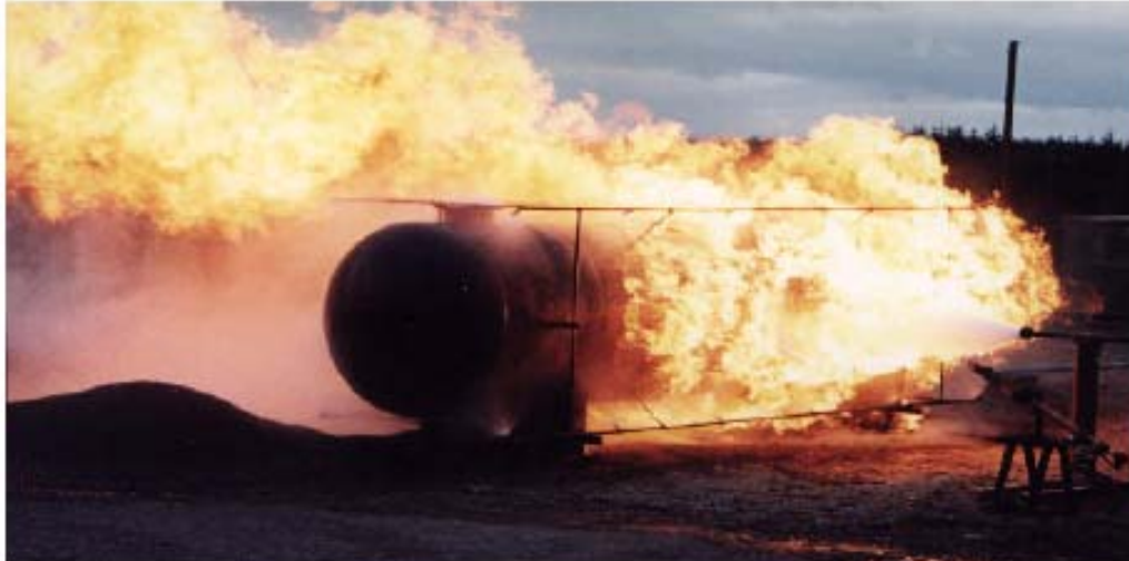
Figure 3.7: Jet fire test with deluge [92]
