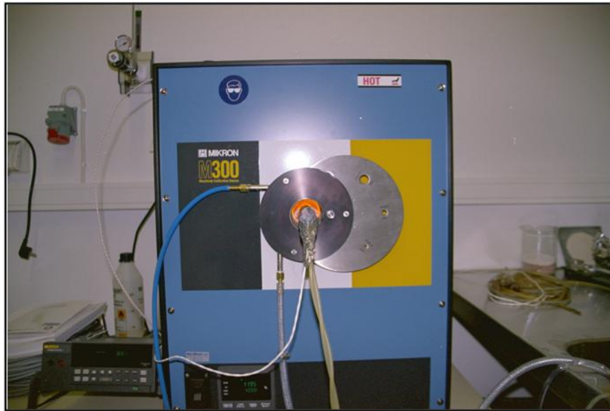
Figure 4.32: Heat flux gage in position during a calibration
