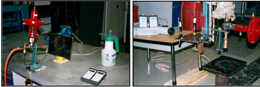
Figure 4.3: Bench scale steel plate in upright (left) and horizontal position (right)
