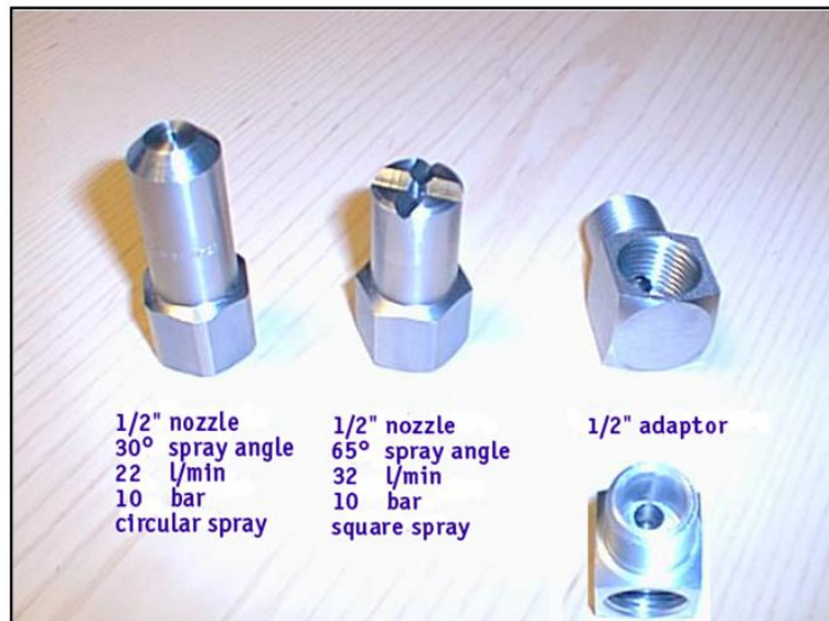
Figure 4.21: Spray nozzles and positioning adaptor
