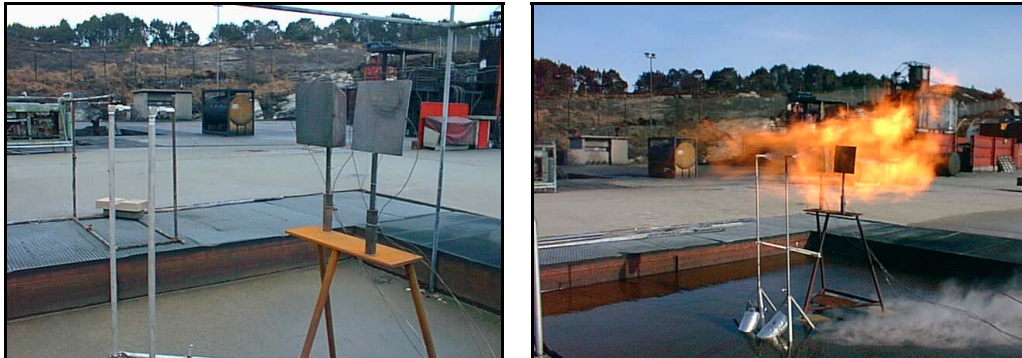
Figure 4.18: Setup with deluge inside flame, prior to (left) and during an experiment (right)
