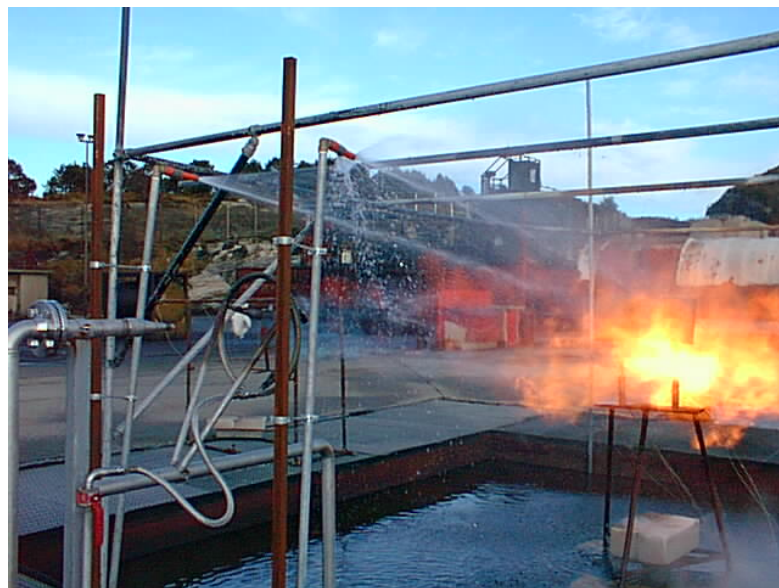
Figure 5.19: Uneven deluge due to nozzle deformation, nozzle 1 on right side
