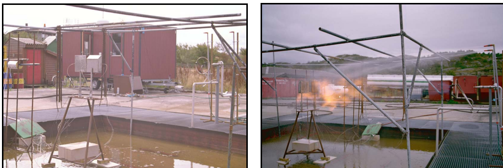
Figure 4.17: Setup with deluge outside flame, prior to (left) and during an experiment (right)
