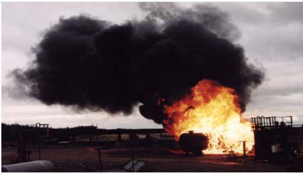
Figure 3.6: Jet fire test without water spray [92]
