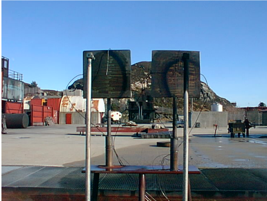
Figure 5.25: Areas showing sign of dry patches on both surfaces, photo taken after experiment
