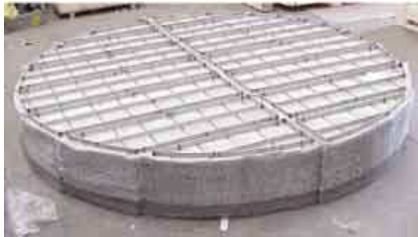
Figure 1.4: An industrial wire mesh demister [32]
