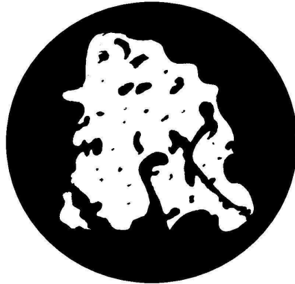
Figure 3.2: Re-entrainment in an annular flow
