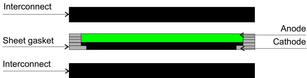
Fig. 8.2: Exploded view showing details of cell sealing (not to scale).
