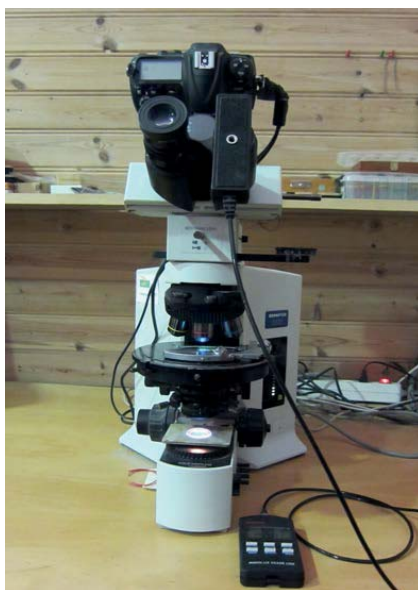
Figure 2: Microscope with Mavolux luminance sensor mounted in one eyepiece.
