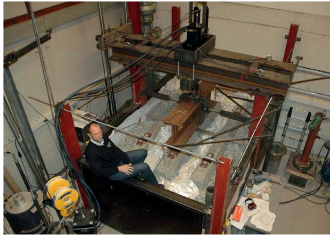
Figure 2: Full scale rail track model test setup for cyclic loading.
