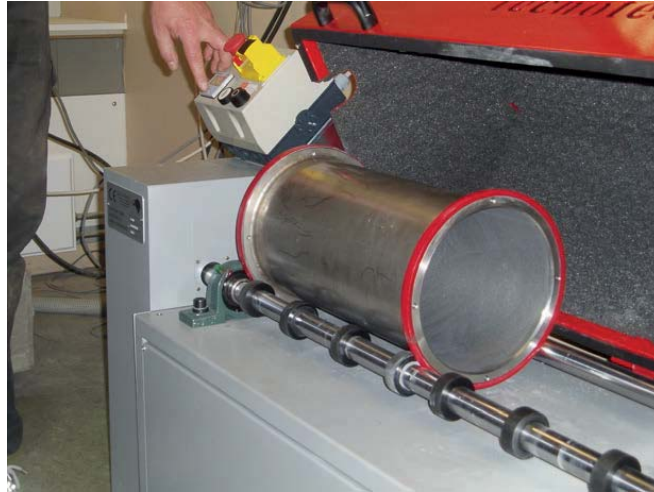
Figure 2.7 The micro-Deval test cylinder for fraction 31.5/50 mm ballast.
