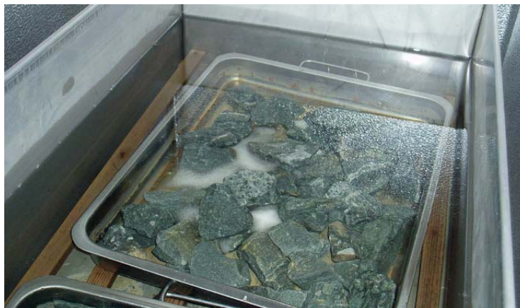
Figure 4.20 Thawing phase of the test. Test material was soaked in water during both freezing and thawing.
