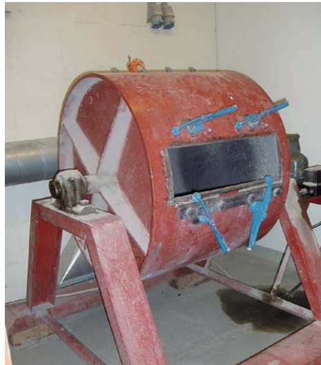
Figure 2.5 The Los Angeles abrasion test drum without cover used for both fraction 10/14 and 31.5/50 mm. Interior diameter is 71 cm.
