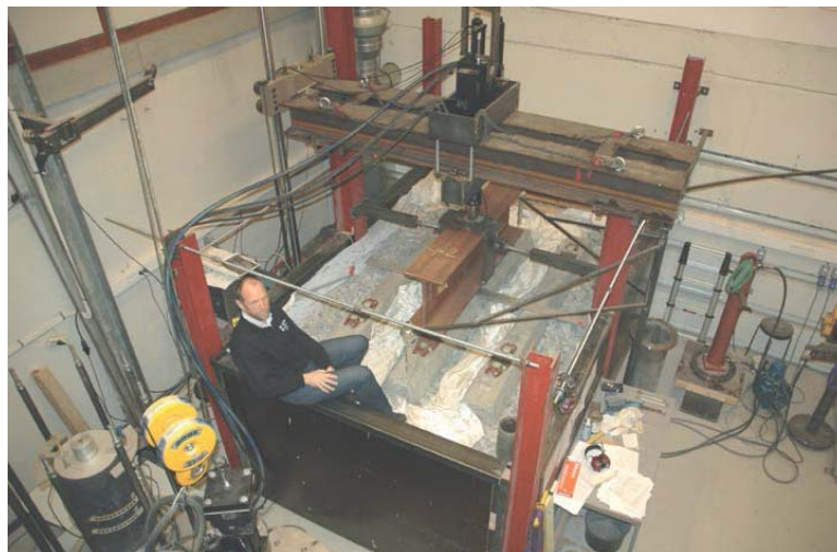
Figure 2.22 Full scale rail track model test equipment for cyclic loading simulating train traffic and tamping.
