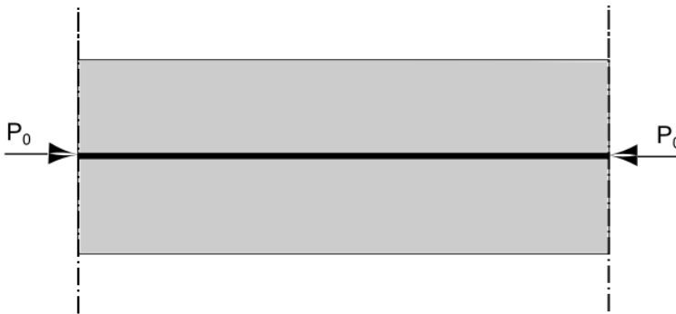
Figur 3.3: Forenklet rettlinjet spennarmering
