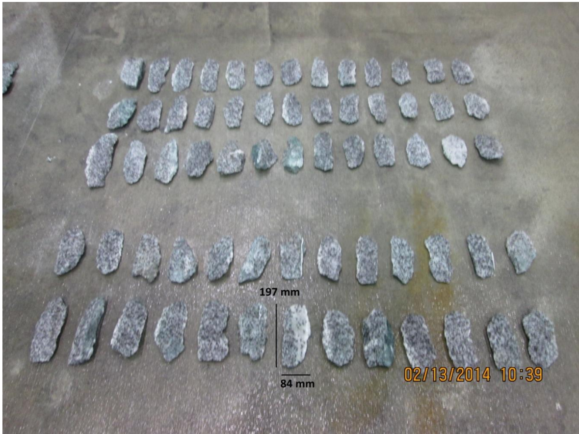
Figure 5.26: Rock chips picked during RPM trial - 3300 PSI. RPM levels from top row to bottom: 10, 9, 8, 7, 10. The mean thickness of the bottom row was 28.2 millimeters.
