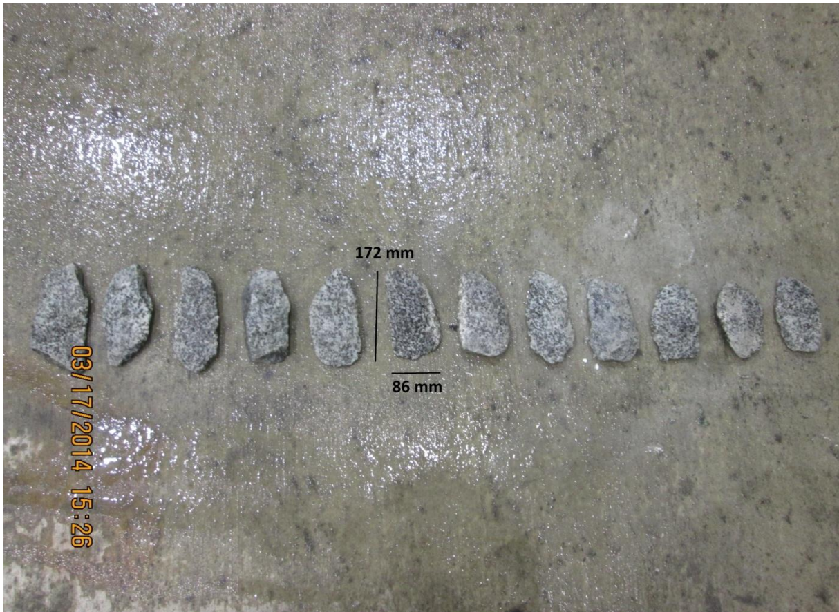
Figure 5.40: Rock chips picked during RPM trial - 2700 PSI. RPM level 10. The mean thickness of the chips was 30.2 millimeters.
