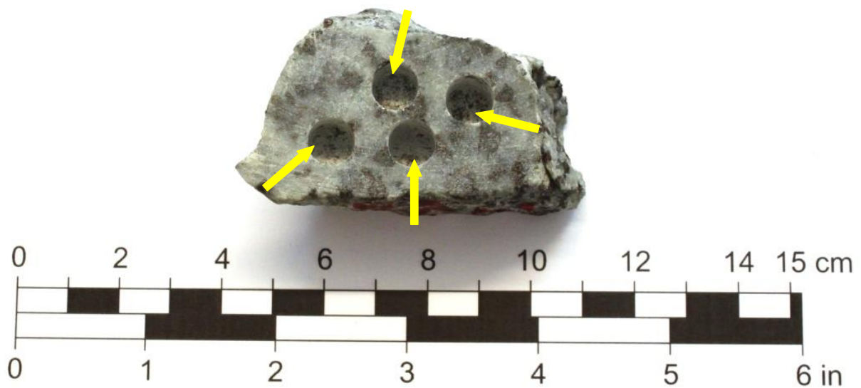
Photo of the Sievers' J (SJ) specimen subsequent to completed testing. Yellow arrows indicate the position of the drillings.
