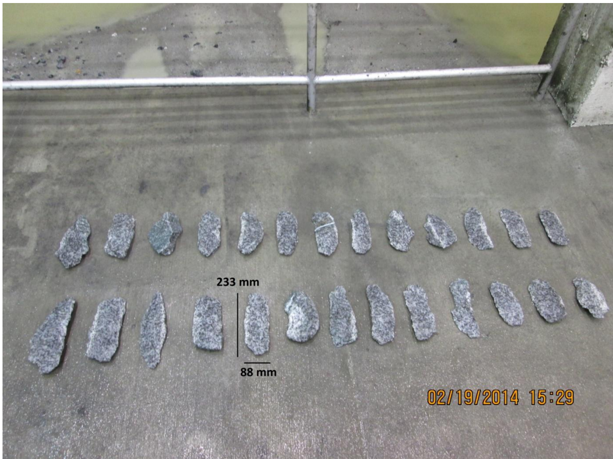
Figure 5.33: Rock chips picked during RPM trial - 3000 PSI. RPM levels from top row to bottom: 10, 9. The mean thickness of the bottom row was 25.8 millimeters.
