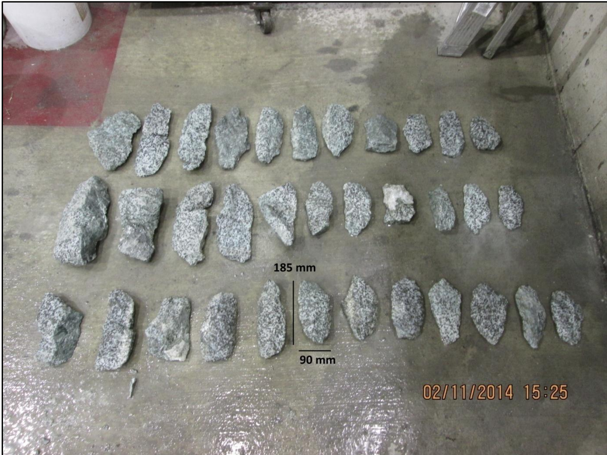
Figure 5.13: Rock chips picked during penetration test 1. Thrust levels from top row to bottom: 3100 PSI (325 kN/c), 2550 PSI (268 kN/c), 2700 PSI (284 kN/c). The mean thickness of the bottom row was 32.2 millimeters.
