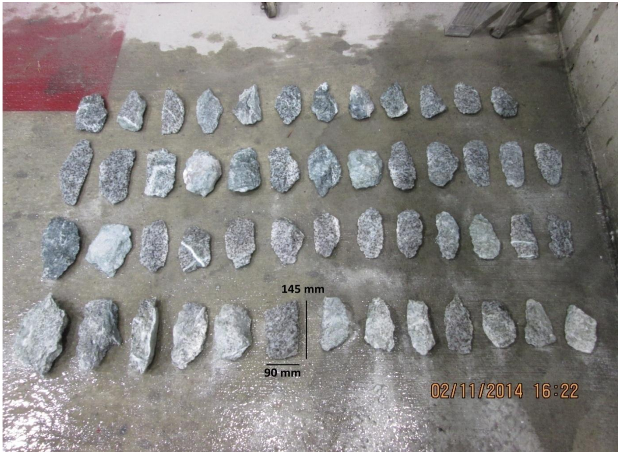
Figure 5.19: Rock chips picked during penetration test 2. Thrust level from top row to bottom: 3000 PSI (313 kN/C), 2750 PSI (286 kN/c), 2500 PSI (263 kN/c), 3250 PSI (341 kN/c). The mean thickness of the bottom row was 39.6 millimeters.
