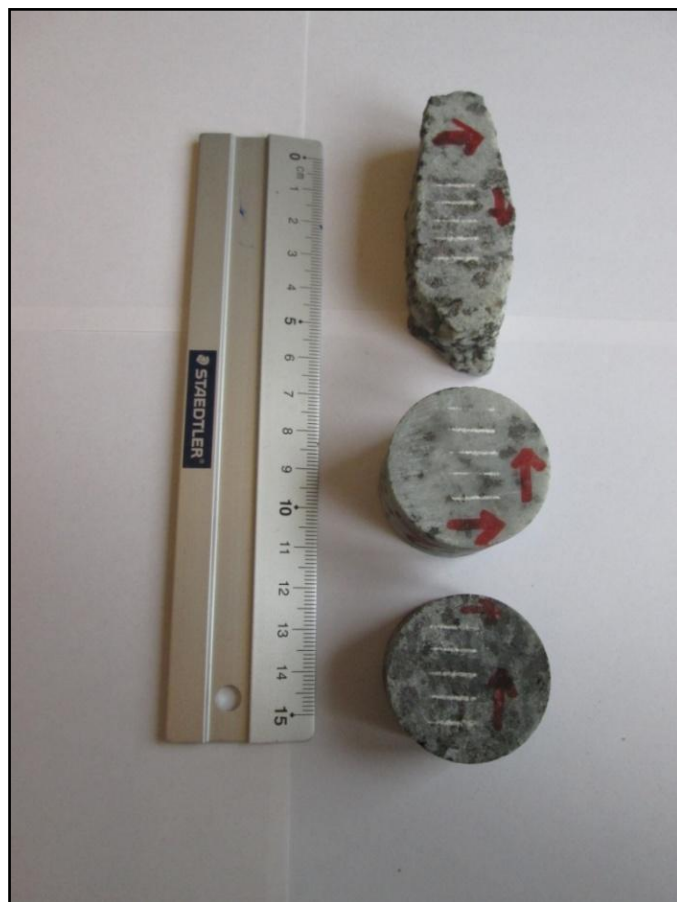
Figure 5.76: Picture of the Cerchar Abrasivity Index samples after testing
