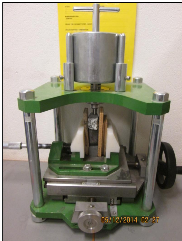
Figure 4.13: Test Apparatus used for the Cerchar Abrasivity Index Testing
