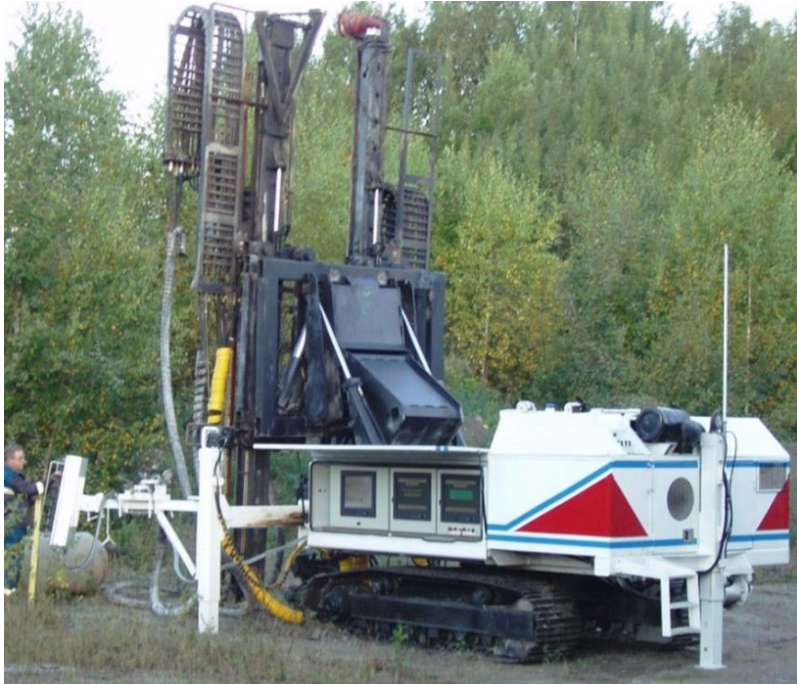
Figur 5-32: Dieseldrevet borerigg. (Jetgrunn, 2014)
