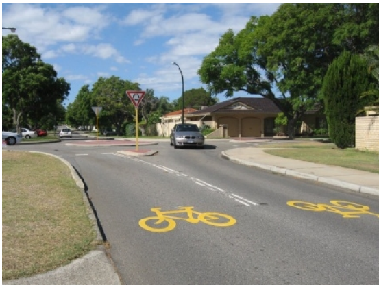
Fig. 13. – Roundabout with advisory lane markings 14
