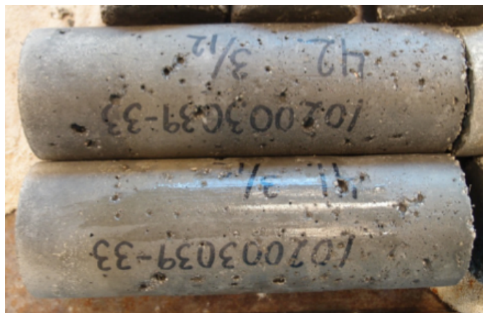
Figure F.5 Concrete Mix 5 after 300 freeze-thaw cycles
