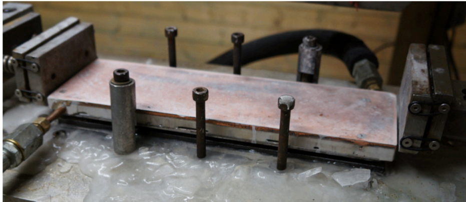
Figure 23 Improved epoxy-copper bedding
