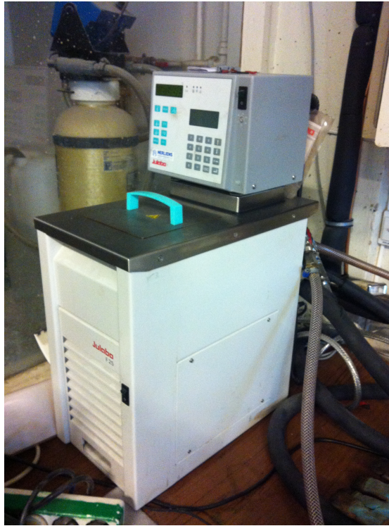
Figure 25 Julabo 2000 heating circulator
