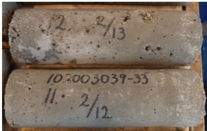
Figure F.2 Concrete Mix 2 after 300 freeze-thaw cycles
