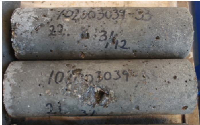
Figure F.3 Concrete Mix 3 after 300 freeze-thaw cycles
