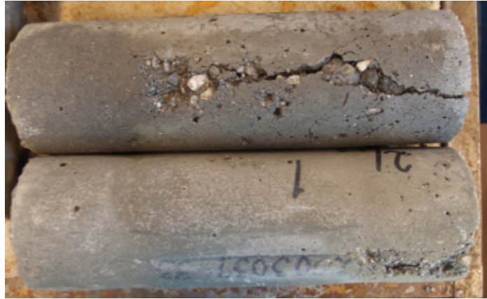
Figure F.1 Concrete Mix 1 after 300 freeze-thaw cycles
