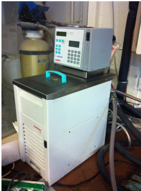
Figure B.5 Julabo 2000 heating circulator
