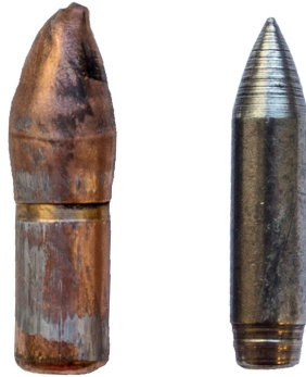
Figure 4.10: Projectile that passed through HAZ with brass jacket intact compared to the steel core.
