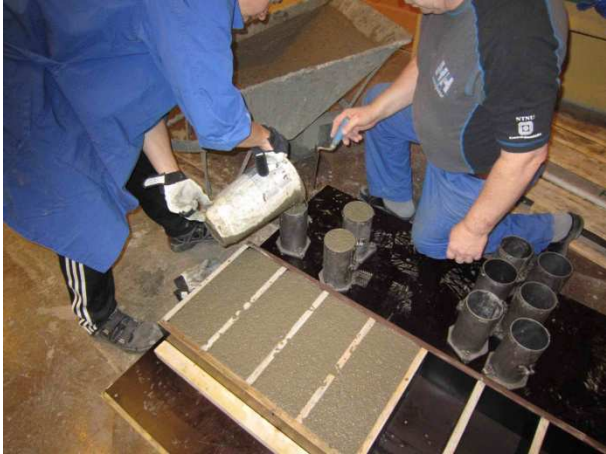
Figure 3.5 Casting of unreinforced LWAC prisms and cylinders
