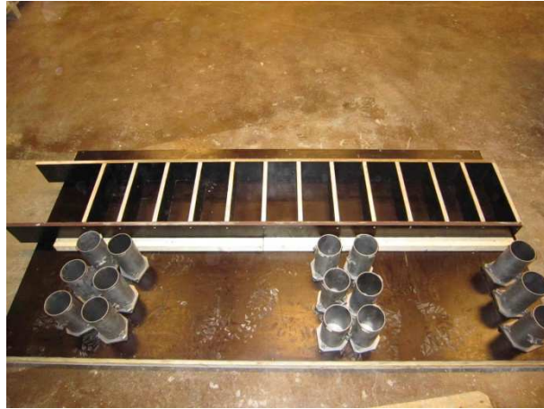
Figure 3.3 Formwork for prisms and cylinders
