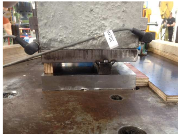
Figure 3.8 Eccentricity at bottom
