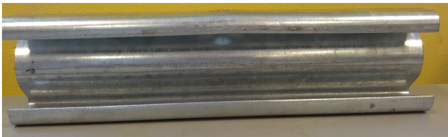
Figure 5.14: Deformed \Sigma -post from test two in the 0° configuration
