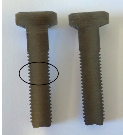
Figure 5.15: Bolt cut in half in preparation for the hardness test
